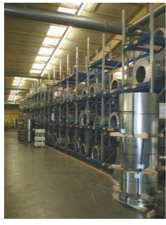
We are mainly working with flat products such as sheet metal and tapes. Most of the material has been galvanised DX 51 D+Z with a pressure by load of approx. 150 gramme per  $\rm m^2$ .
