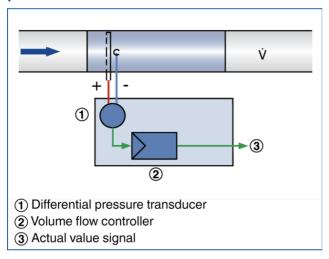
$\label{lem:definition} \mbox{Differential pressure sensor for the measurement of non-contaminated supply air.}$
